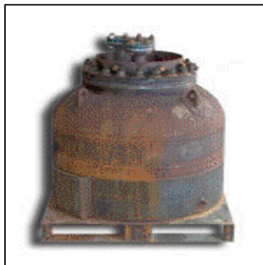
Chemical tanks with lead lining
